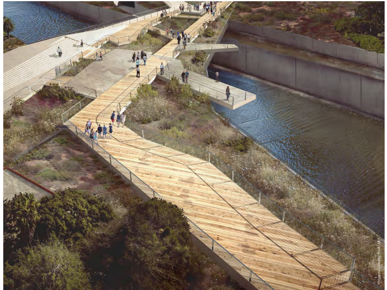
▶ Cantilever deck rendering featuring two deck locations and integration into boardwalk-type pedestrian path.
