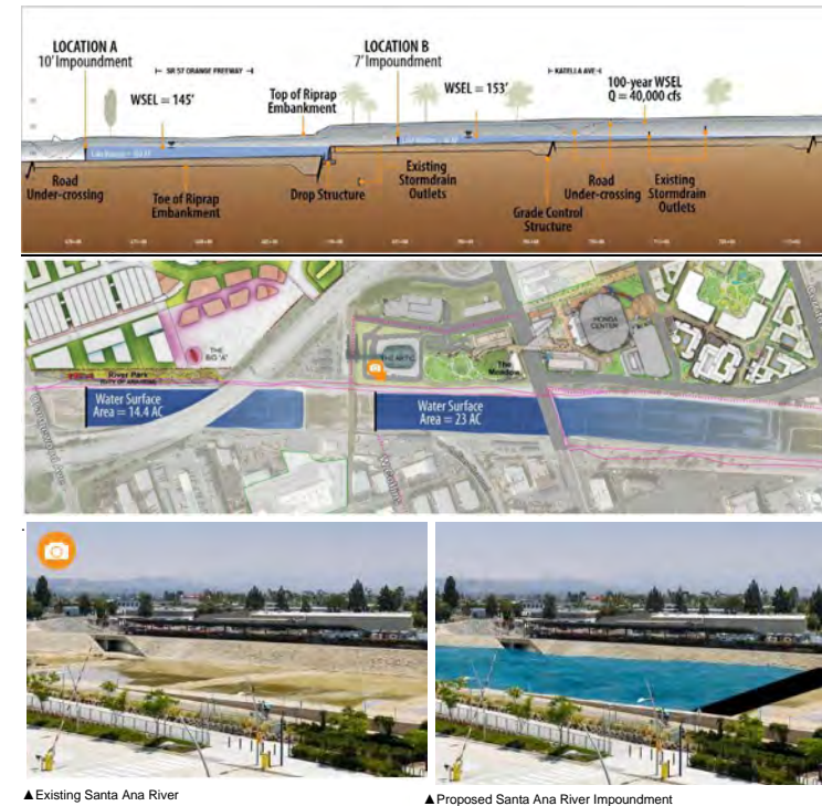
Figure 3: Plan & Profile and Conceptual Render of Potential Impoundment Location
