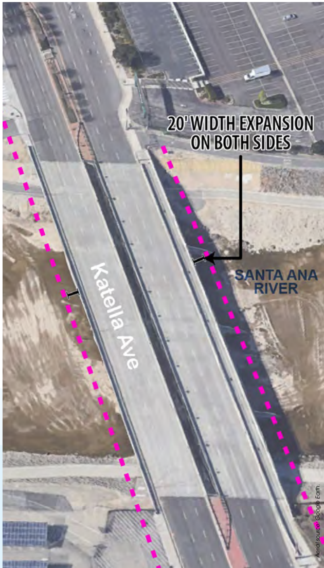
▲ Photos show the aerial plan view extents of a 20-foot widening on both bridges.
