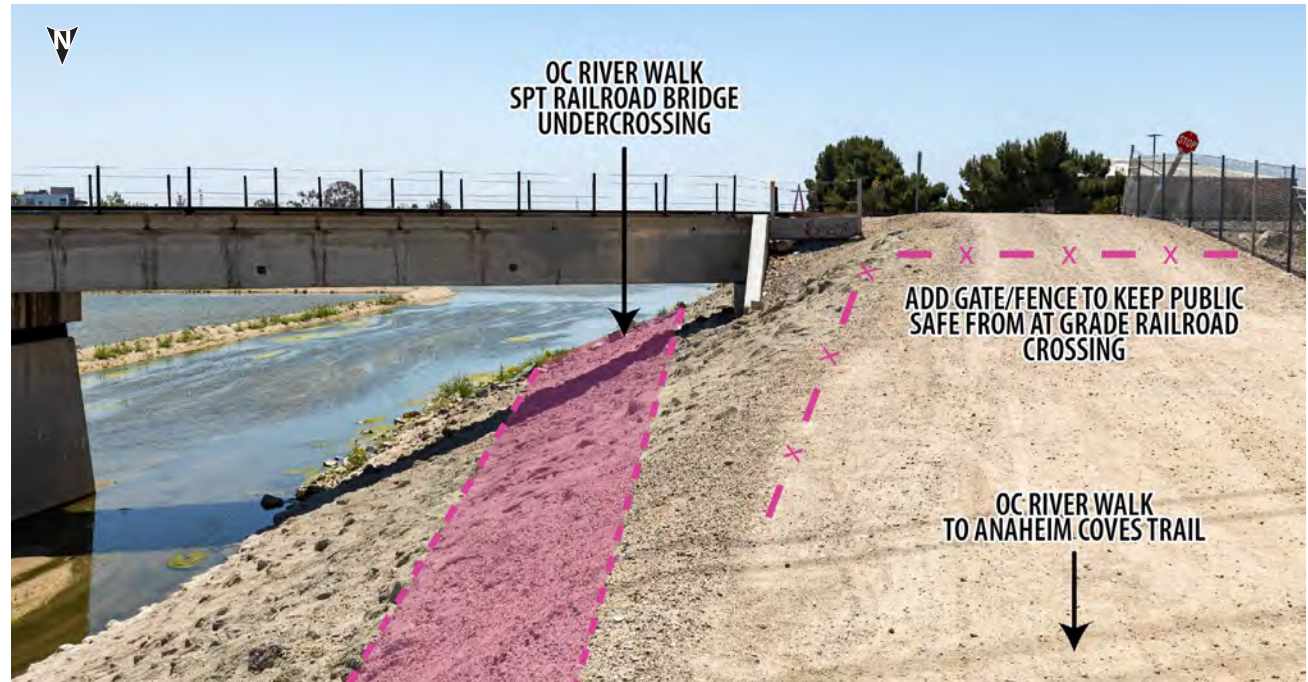
▲ On west bank, looking south at the proposed SPT undercrossing footprint and alignment. A similar at-grade gate & fence to be installed on the North side, identical to the South side.
