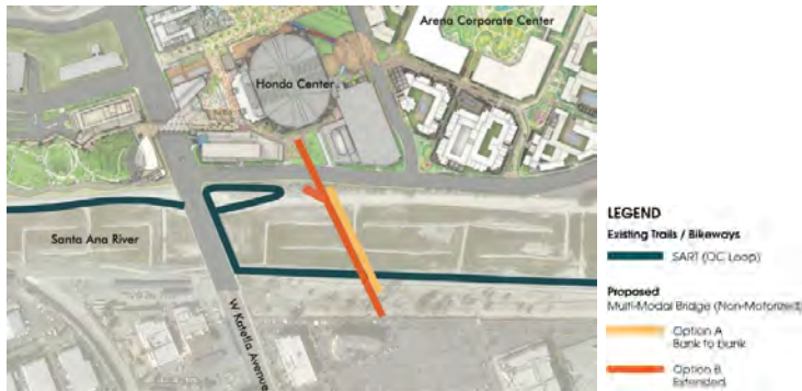
Figure 4: Plan View of Proposed Non-Motorized Bridge Options
