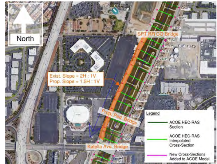
Figure 14: River Embankment Slope Modification (2:1 to 1.5:1)
